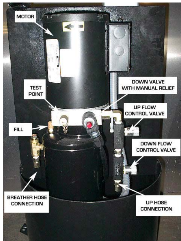
Figure 1-2c: Hydraulic Unit Side View
